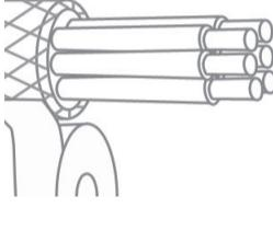
**EN** Make sure to use shielded twisted-pair cable. Strip cable 55 mm, strip the wire ends 8 - 9 mm and put the shield over. Insulate the whole shield with tape. Contact between shielding and board may cause substantial damage to the unit. Make sure that the correct wire pairs are twisted together when wiring (I. CAN high - CAN low, 2. GND - VDC).
